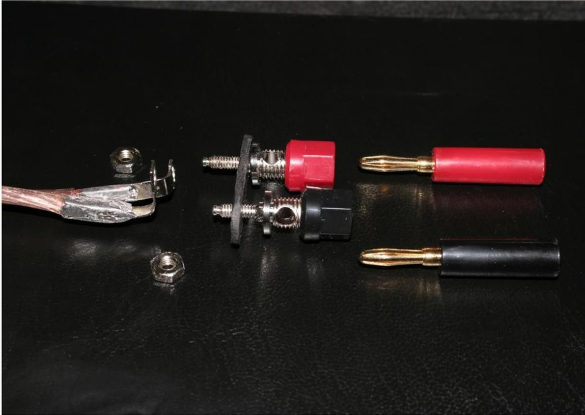
Connectors' installation is simple. I drilled two holes in place where I considered the connectors most convenient. I soldered copper wire to the connectors and installed them. I used  $2 \times 5 \text{mm}^2$  twin-lead cable as the wire should be as thick as possible to reduce resistance. I sealed the connectors inside of the box with bitumen sealant so that they resist vibrations. As I didn't want the cable to just lay at the bottom of the box, I stuck it into a layer of bitumen.
