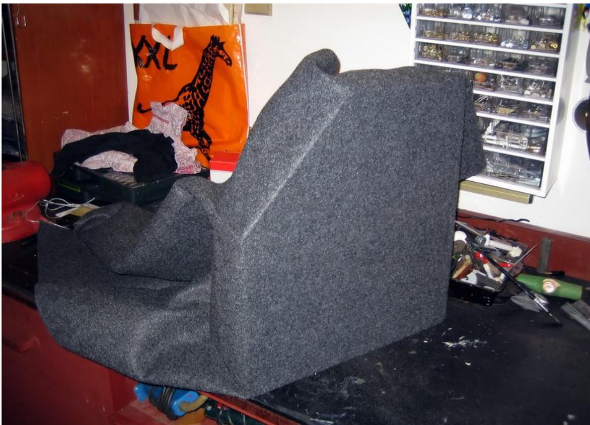
When the glue dried out I cut the hole for the speaker with a sharp knife.
