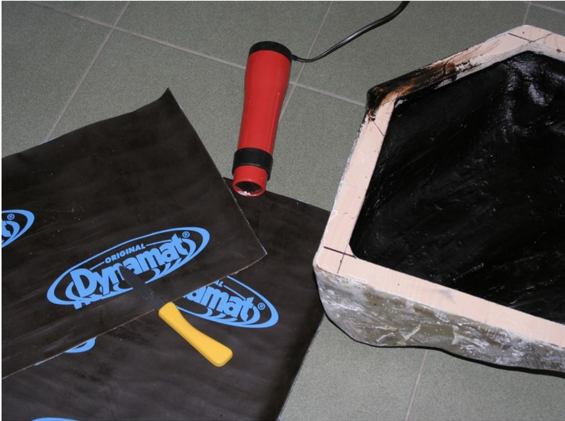
I had some rest of Dynamat sound damping I used previously during my audio installation, so I decided to stick a layer of Dynamat too. It was not exactly necessary but it won't harm either 😊.
