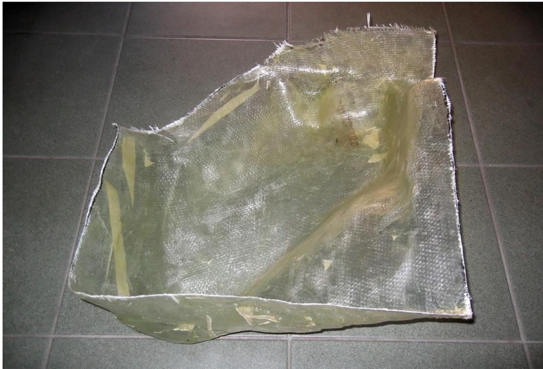
With electric saw I cut the sides to have (more or less) straight edges.
