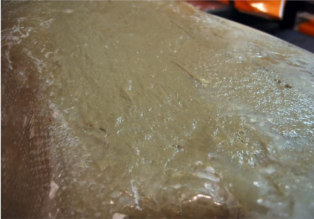
Another close-up of the fiberglass body filler I used on the back of the box that has to be smoothed.
