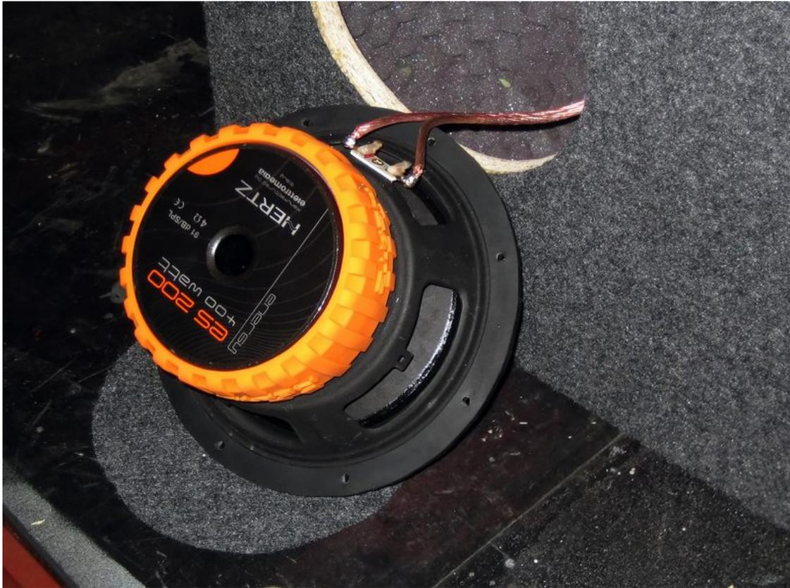
Speaker installation is quite easy and you can't do much wrong. I soldered the wires to the speaker as I don't expect to take the speaker out often (if ever). Simple connectors can be used as well, but if they don't fit tight the vibrations might make them loose after some time.
