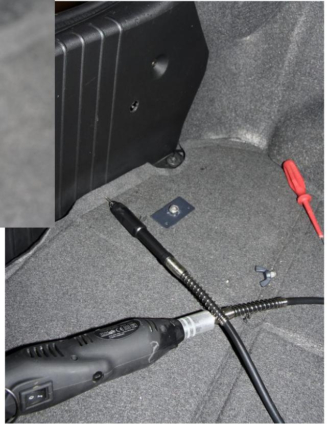
I cut holes into the boot trim to host the screw nuts. I cut them a little larger, so that I had freedom to fit fixing points exactly on the spot where I needed them.
