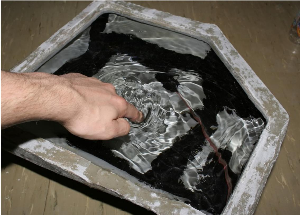
When you build a subwoofer, you have to know its volume to choose appropriate speaker for the enclosure you have. Or you can choose the speaker first, and build an enclosure with an appropriate volume to its characteristics. When building a box, it is easy to calculate the volume, but with curved custom shape, it is almost impossible. As I wanted to know the volume of the box I have built I could come to only idea: fill it up with water ☺.
