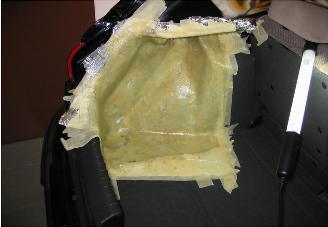
This is how my fiberglass box looks like while drying. Three hours later, I could easily take the molding out and to my surprise I could peel most of the paper tape down quite easily.
