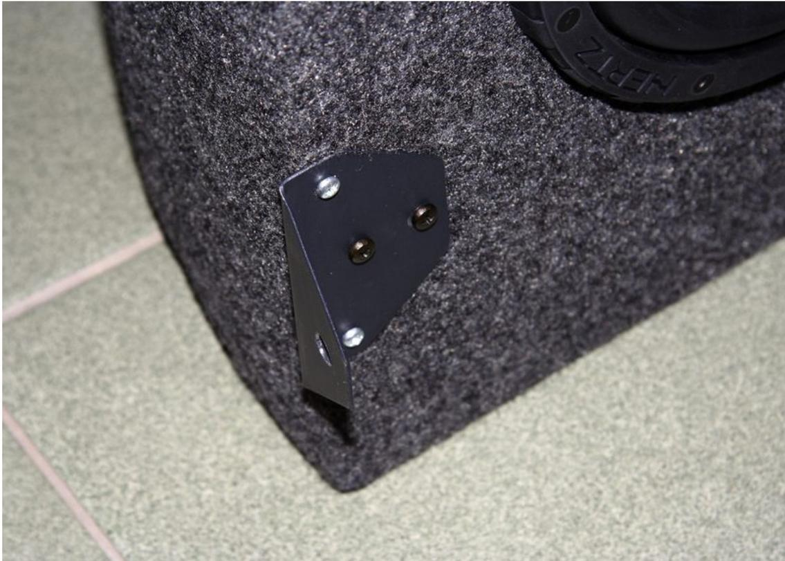
Subwoofer mountings on place. One of them is screwed in wooden front panel, second one is held by screws in fiberglass on the box side. I used more screws, to lower the stress put on fiberglass material. I am sure that two screws would be enough to hold the box in place, but I have always tendency to come it strong.
