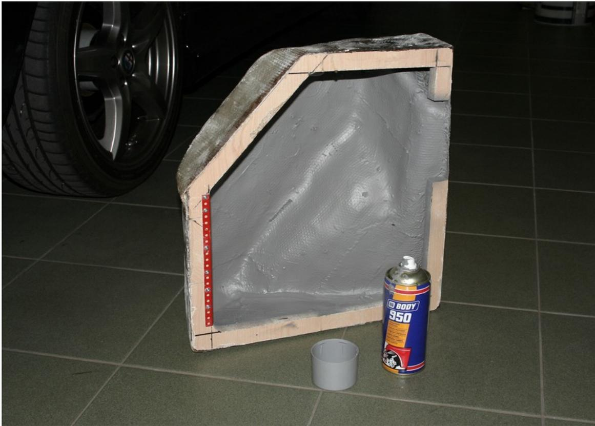
I sprayed the inside of the box with spray used for underbody (chassis) protection. If you are very serious in car audio you can use so called “noise-killer” spray available in audio shops, but according to the information on my spray, this one has the same composition (asphalt and bitumen) for 1/4 of the price.
