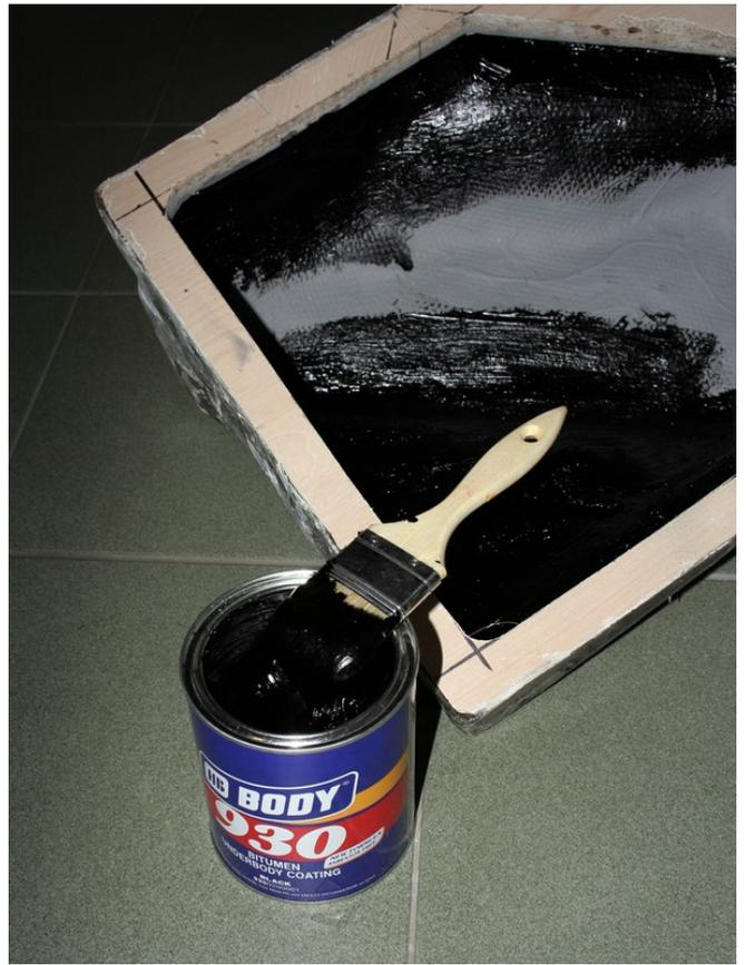
As the subwoofer walls have to be as rigid as possible and resistant to vibration with good sound damping properties, I decided to paint it from the inside with bitumen underbody coating. Though it is quite thick material, I was still able to paint it with a normal brush. Though it dries very quickly for the touch in thicker layer it is quite delicate. Because of this I let it dry for a week.
