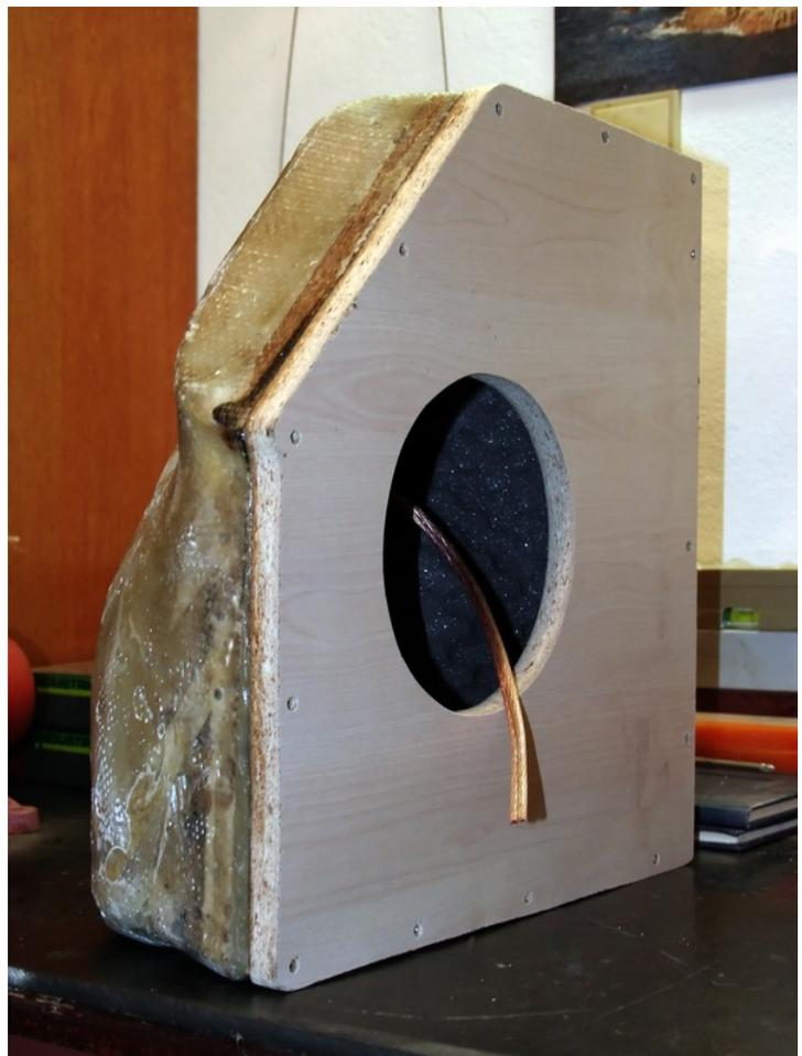
My work is at least starting to look like a box 😊. Not a nice one, but this can be still improved. I have to smooth the surface roughness with a filler. I used fiberglass filler for places where I needed thicker layer as the glass fibres inside the filler make it very resistant and it doesn't crack. For thin layers and final finish I used polyester fillers as they are easier to smooth with a sandpaper.
