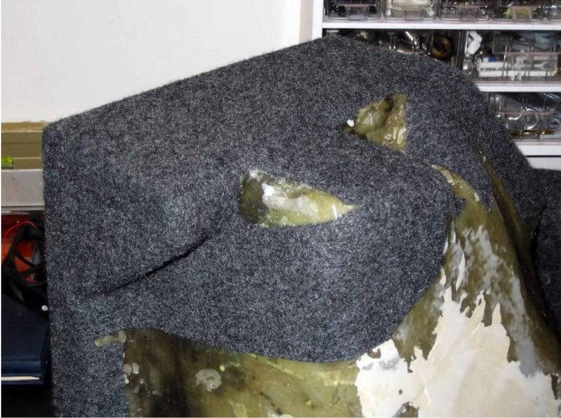
This was the most difficult part of the box to upholster because of its shape. It can hardly be covered with a single piece of carpet. I had to work with 4-5 smaller pieces I cut separately.
