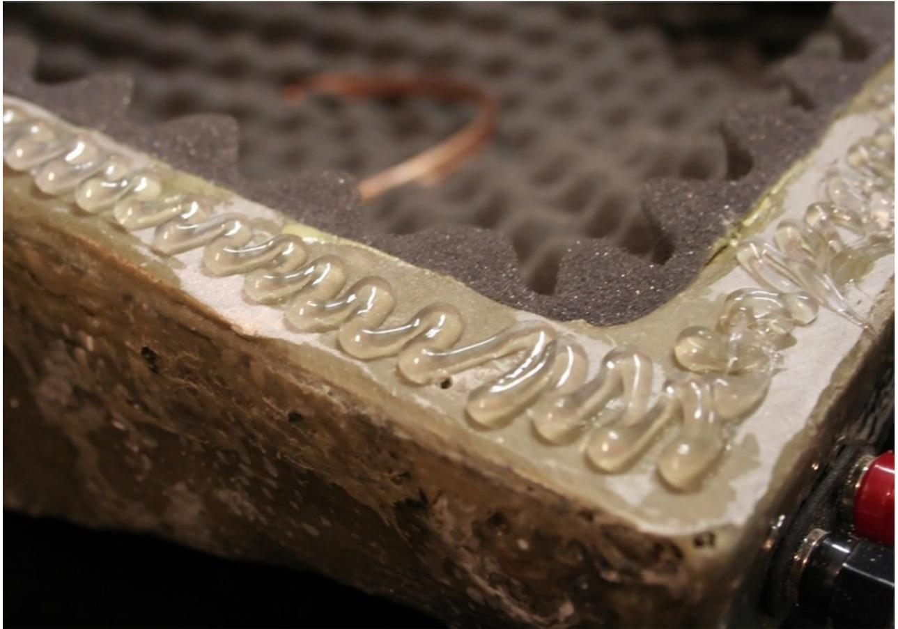
I connected the front and back of the box using universal transparent silicone and 13 screws. The good thing is that the box is completely sealed now, but it can not be disassembled in the future. After it is smoothed and upholstered it is even impossible without destroying it. But for me it is not a problem as this was the plan. It would be much more difficult to build a box that could be opened.
