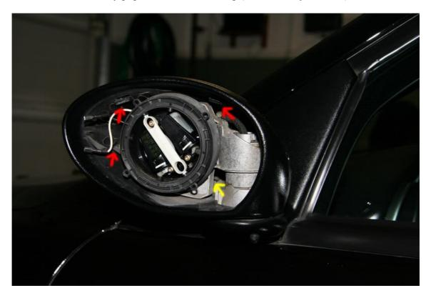
5. The cover comes out by sliding it forward. If your car is not brand new, the cover will be probably "glued on" by water and dirt that has progressively got between the frame and cover. I was surprised how much force I had to use to slide the cover (be sure the clips are released and didn't pop back in as in this case force will not help).
