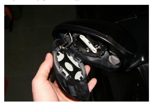
4. The cover holds on 4 clips. Three of them are well accessible (red arrows) and one (yellow arrow) is accessible only if you take apart all the mirror adjustment assembly. But this is not necessary to do as if you release the three and if you apply reasonable pressure on the cover, the fourth will eventually pop out without breaking (at least in my case did).
