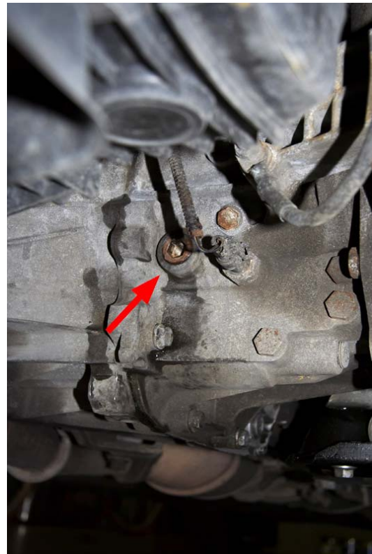
Drain plug (pictures were taken after the oil change, that's why the gearbox is dirty of oil)
