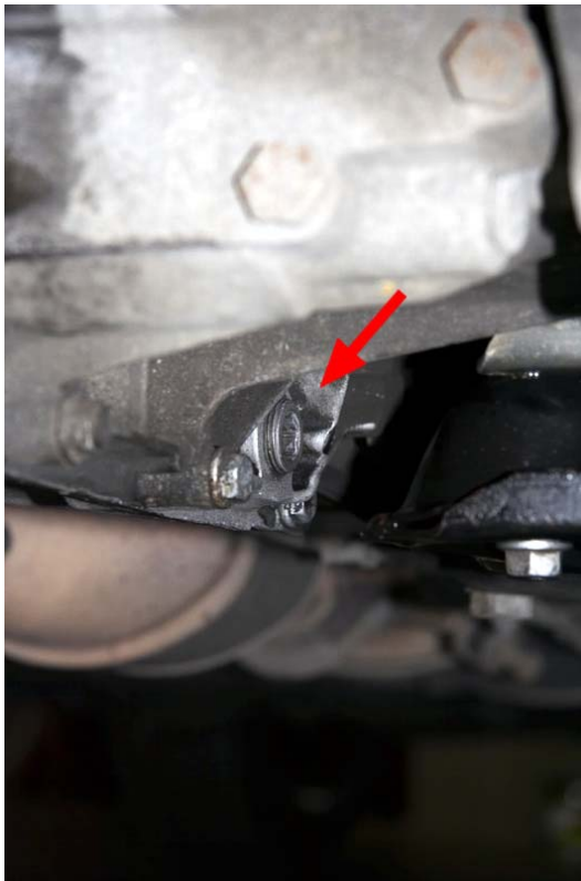
Drain plug (pictures were taken after the oil change, that's why the gearbox is dirty of oil)
