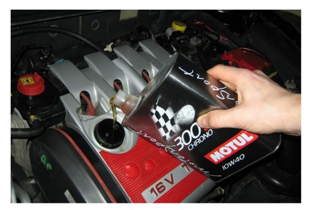
Close the oil filler cap and start the engine. It might happen that you will see a "low oil pressure warning" at startup, but this should go off quickly. Let the engine idle for a minute or two, turn it off and wait for a few minutes. Check the oil level on the dipstick and fill up if necessary.
