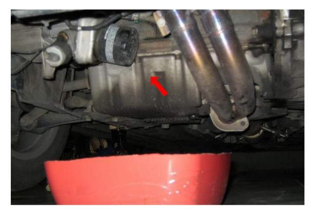
9. Unscrew the oil filter. It might be doable by hand but it is much easier with the right tool. There are many sorts of oil filter keys widely available and they are usually very cheap.
