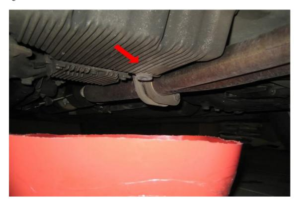
Put a suitable container (min 5 ltr. capacity, flat enough to fit under the car) under the drain plug. Unscrew the plug and let the oil drain out. Wear glows as the sump and oil are very hot. Lower the car if you lifted only one side so that the car stands flat and all oil can flow out.
