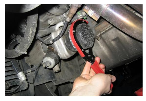
Don't forget to put a container under the filter; there is enough oil in it to make a big mess. Lover the car and let it drain with filter removed.
