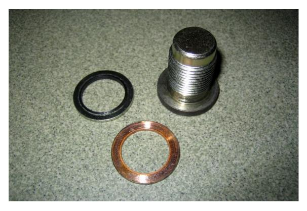
7. Raise the car again and screw the plug back in. The best way is to use a torque wrench set to recommend 22 Nm. This way you know the plug is tight and you don't strip the thread.
